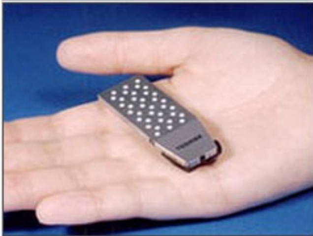
Toshiba- DMFC, 100 mW, 2cc Fuel Tank, 99.5% methanol
